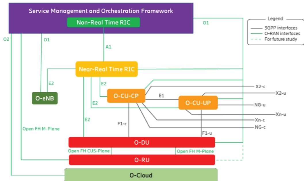
A1 Interface between Non-RT RIC and Near-RT RIC to enable policy-driven guidance of Near-RT RIC applications/functions, and support AI/ML workflow - O1 Interface connecting the SMO to the Near-RT RIC - O2 Interface between the SMO and the O-Cloud - E2 Interface connecting the Near-RT RIC or more O-CU-CPs/UPs/DUs/O-eNBs - Open Fronthaul CUS-Plane Interface between O-RU and O-DU - Open Fronthaul M-Plane Interface between O-RU and O-DU and between O-RU and SMO.
